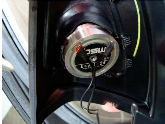
13. Now, snap the upper edges of the tweeter sail back onto the door, and carefully note how the rear edge of the tweeter pod needs to hook into the groove before you attempt to snap the pod into place. The BSW tweeter wire will plug into the connector attached to the midrange speaker when you're reattaching the door panel. Don't worry about the factory tweeter plug.
