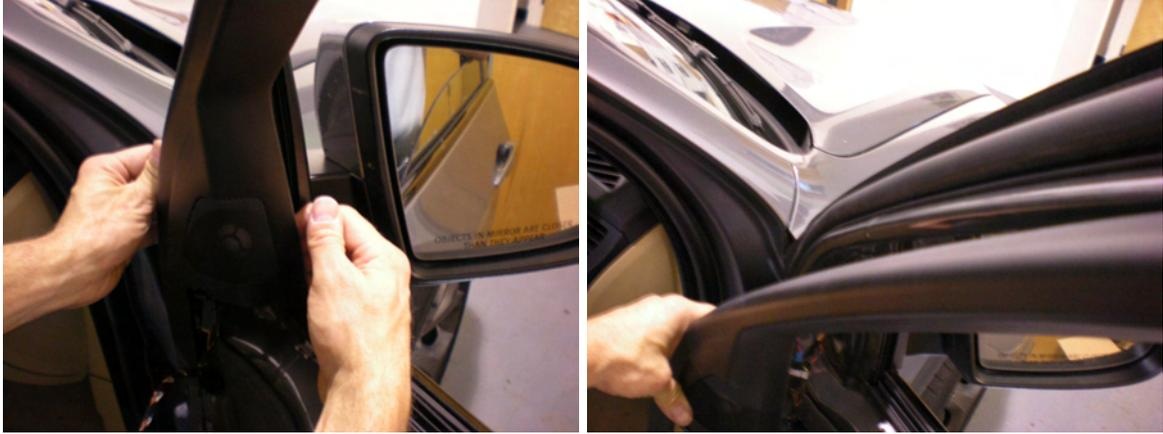
12. Pry off the foam, and with the factory tweeter exposed, remove it using your angle pick tool. Carefully pry out at the attachment points, and the tweeter will free itself. Snap the new BSW tweeter into place, reinstall the foam, and voila!
