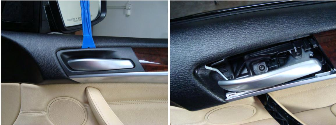
4. Again, using your plastic panel removal tool, carefully pry along the bottom edge of the door pull, as we're going to separate the front of the pull from the rear. Once the initial separation begins, use your hand to remove the rest of the panel. Be firm but gentle in your pulling. Once the panel is removed, two more Torx T20 bolts will be revealed. Remove these, and the panel is ready to be separated from the door itself. See, we told you it was easy!
