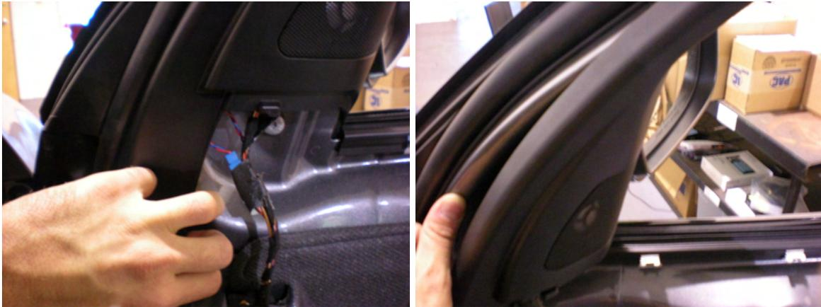
11. With the front edge loose, push toward the rear of the door, freeing the rear lip of the tweeter panel. Now, you can start peeling back the upper section of the tweeter sail so that you can move the pod enough to swap out the tweeters.
