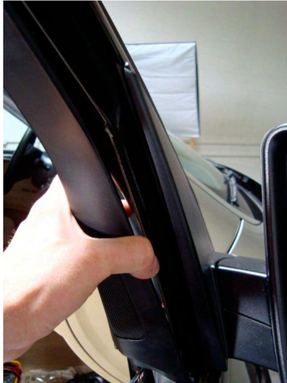
14. With the pod snapped back into place, you're now ready to reinstall the door panel. Don't forget to plug ALL of your connections back into place, as well as your door handle. We recommend starting the attachment process on the top edge of the door panel, and slowly working your way around by ensuring the clips are aligned with the holes in the door before firmly pressing inward, securing the panel for good.
