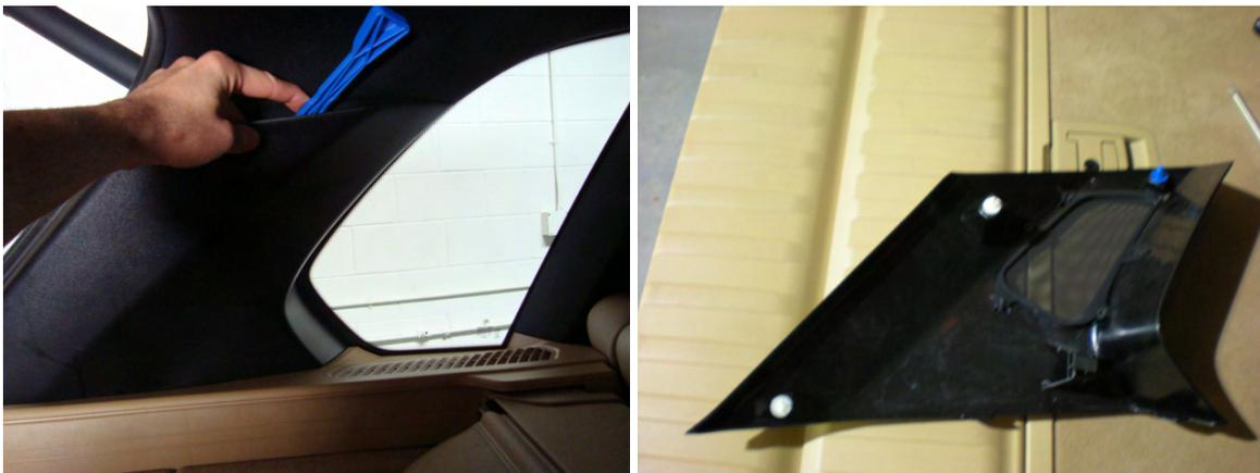
2. With the panel removed, detach the midrange/tweeter pod by removing the three Philips head screws that attach it to the body. Take the pod to your workspace. Remove the three 8mm nuts that attach the factory midrange and pry the factory tweeter out of its housing using your right angle pick. Attach the new BSW midrange to the panel, and snap the new BSW tweeter into the housing (just like the rear door panel). Plug the tweeter into the midrange. Revel in your success.
