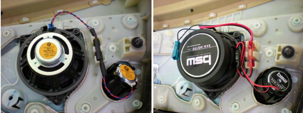
2. The new BSW tweeter will snap right into the housing, and for good measure, you may want to dab a couple of drops of glue to secure the tweeter. Not necessary, but some of us believe there's no such word as "overkill". Plug the tweeter into the midrange.
