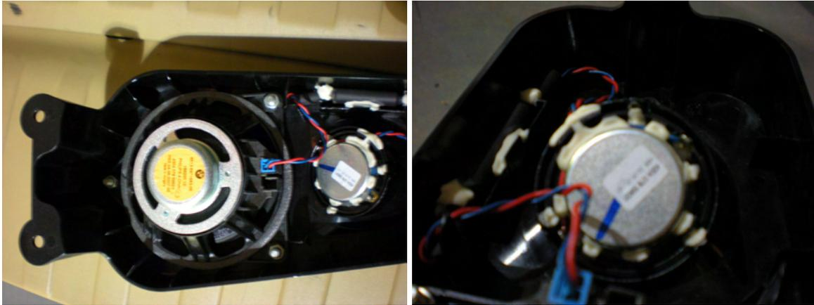
3. Take the housing back to the car, plug in the midrange, and screw the housing back down to the body. Reinstall the panel. Smile.
