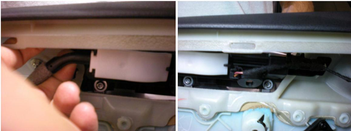
8. With the panel free, take it to your workspace and prepare for the midrange installation. The midrange is attached using three Torx T20 screws. Remove these, and install your new BSW midrange. Simple! Photos on next page.
