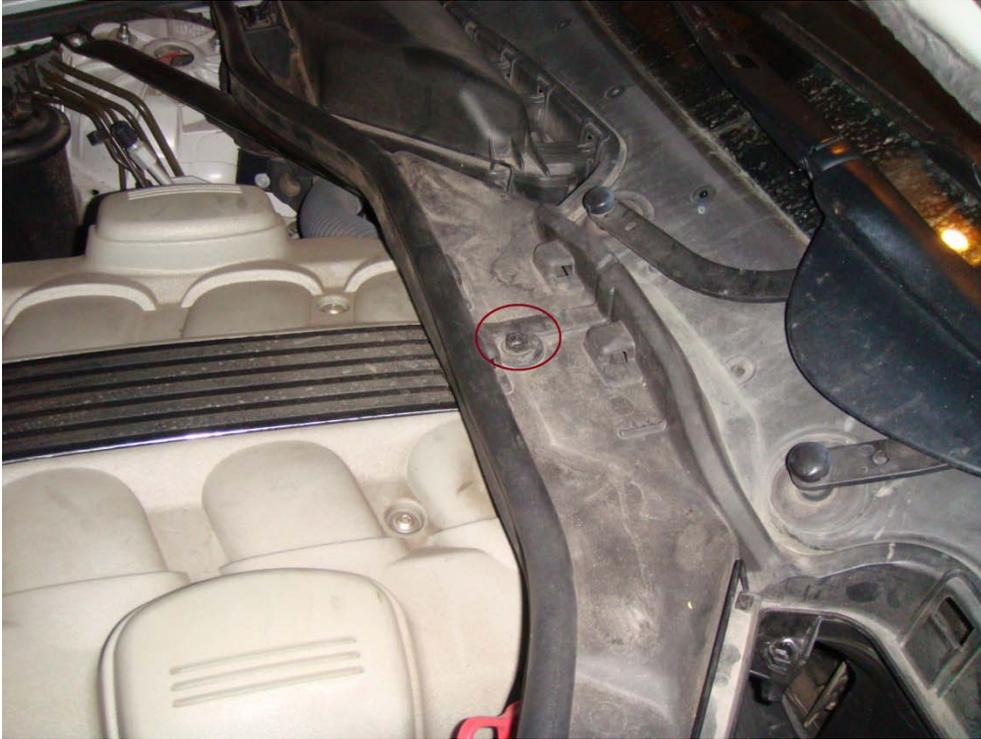
10. Remove trim piece to the left and then lift out the plastic piece.
