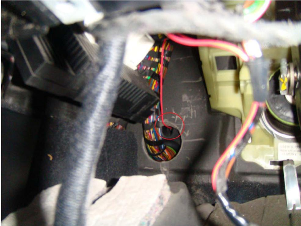
15. With a wire tap, connect the wire to the 12V wire of the foot well light.
