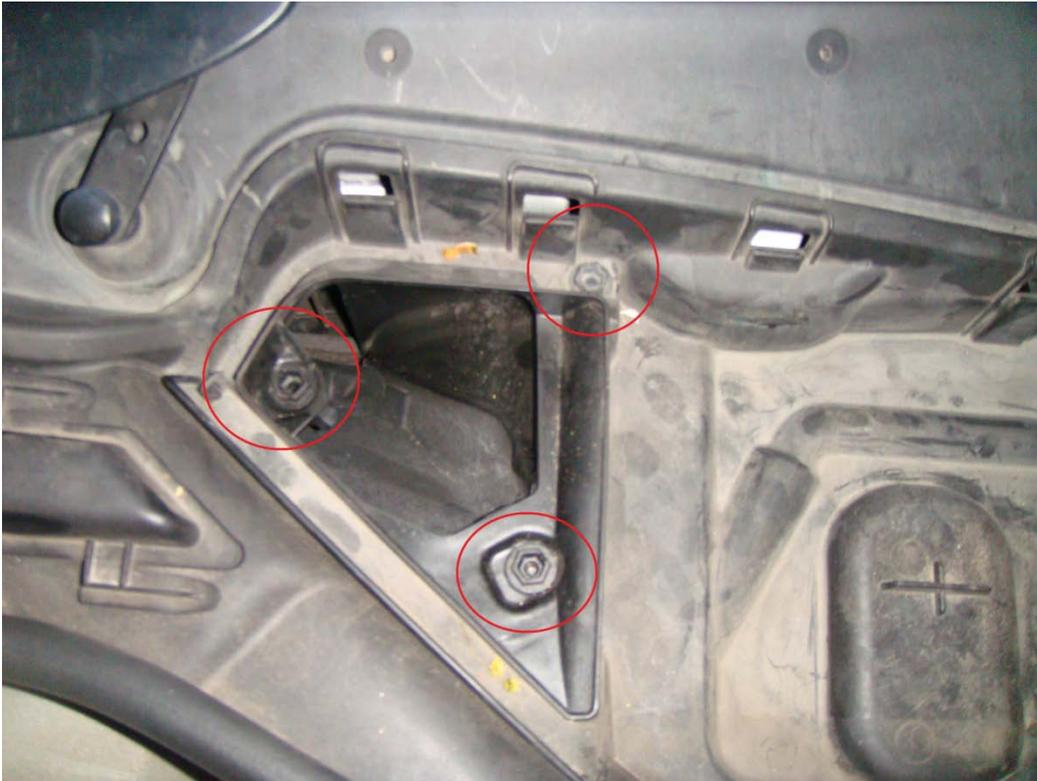
8. Pull up clip and slide towards drivers side then lift up and remove plastic piece.
