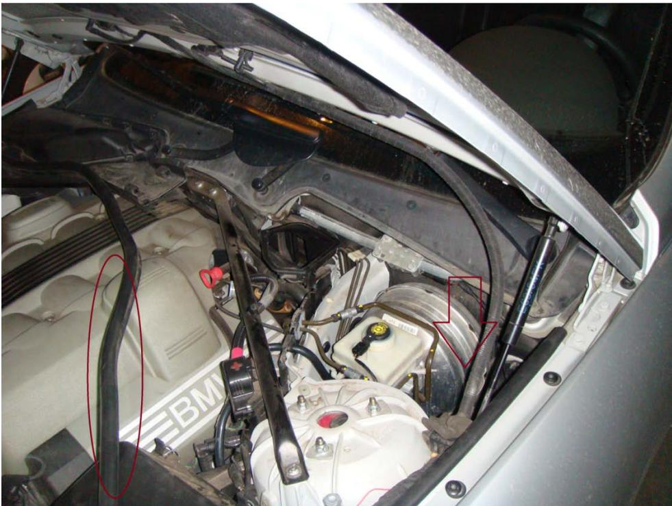
12. Make a small incision to allow for a wire to pass through. (I used a red wire)
