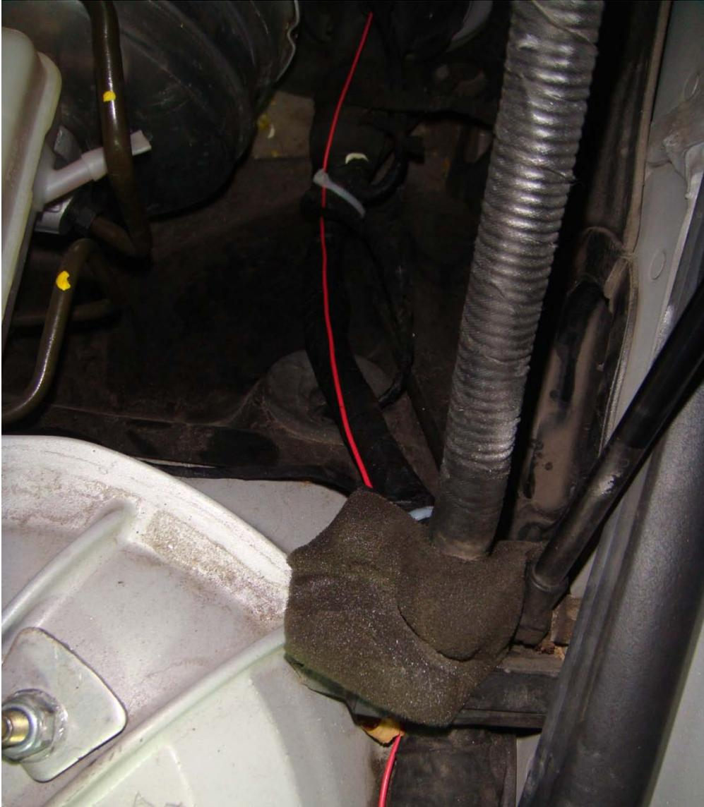
17. Wire tap the wire that was routed to the inside of the car to the 12V wire of the angel eyes.
