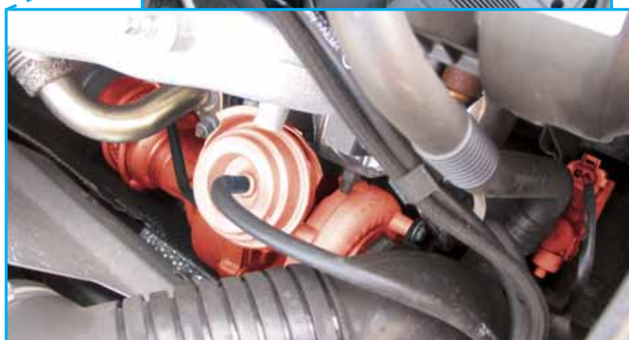
EPW and VTG charger (highlighted in red) in the Audi A4 TDI
