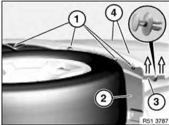
Release screws (1) from wheel arch cover (2) on left/right.
