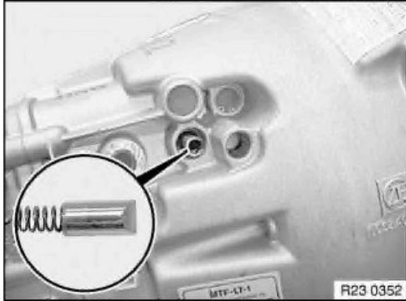
Remove pressure spring and locking pin.
