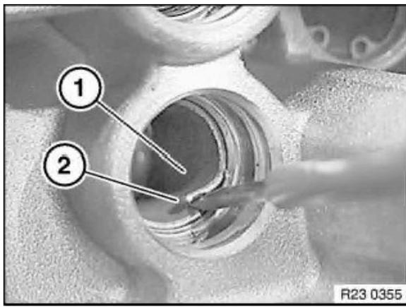
Force open bearing bushing (1) and withdraw using a suitable tool.
