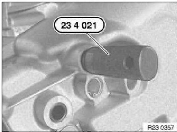
Drive in sealing cap (1) with special tool 23 4 021 .
