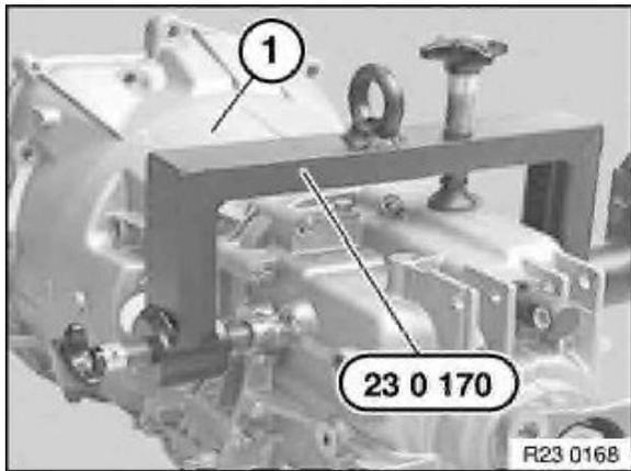
Place transmission (1) with special tool 23 0 170 in assembly stand 00 1 450 .
