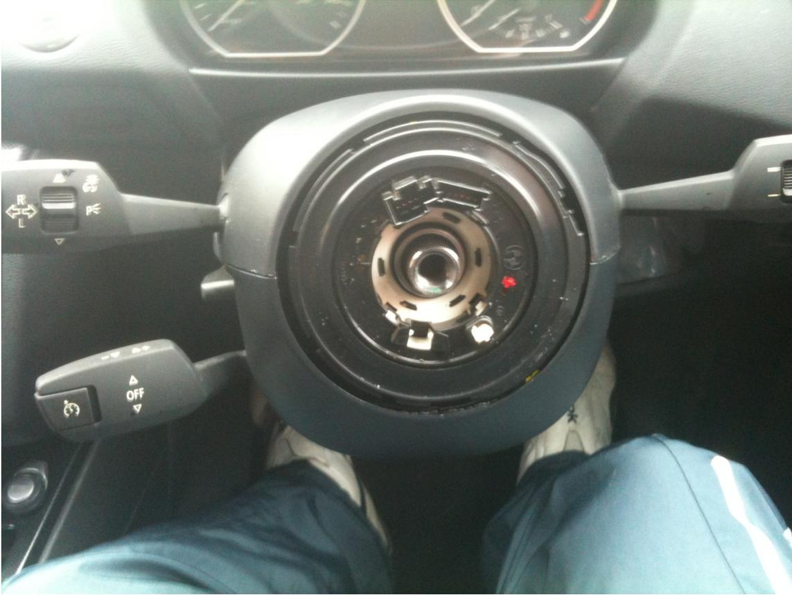
13. Refit steering wheel, making sure that it is correctly aligned as shown in step 6 above. The green marker must be in the centre of the solid bit as shown below.
