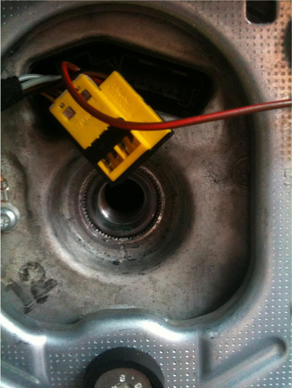
14. Re-fit the 16mm steering wheel bolt and torque to 63nM.
