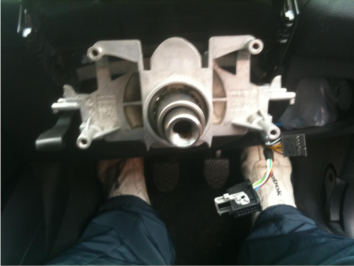
11. Fit new slip ring and reconnect both looms. If you are installing a new slip ring, remove the red coloured transit locking tab first!!!! Re-fit 4 T20 securing bolts
