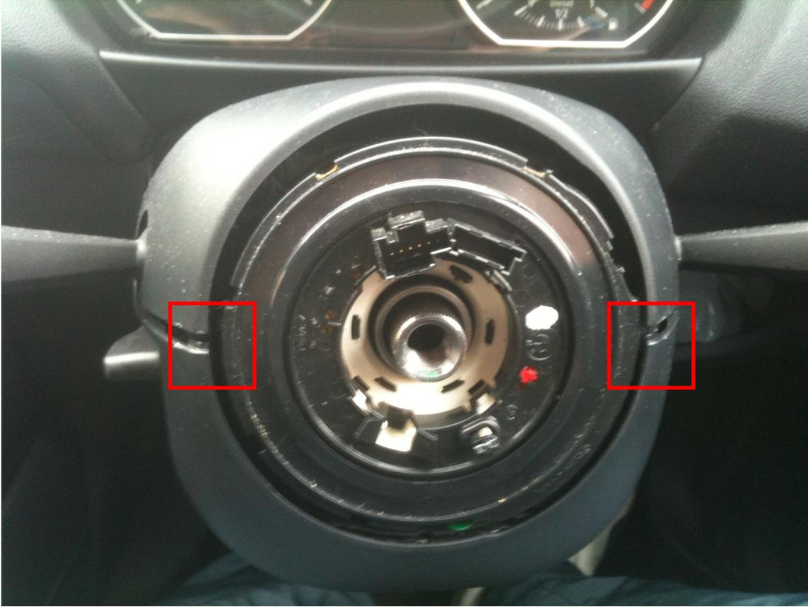
8. You should now be able to raise the top part of the shroud out of the way to expose the rear clips for the lower part. They release by pulling them outboard with gentle pressure in the direction of the arrows. This should allow you to remove the lower shroud.
