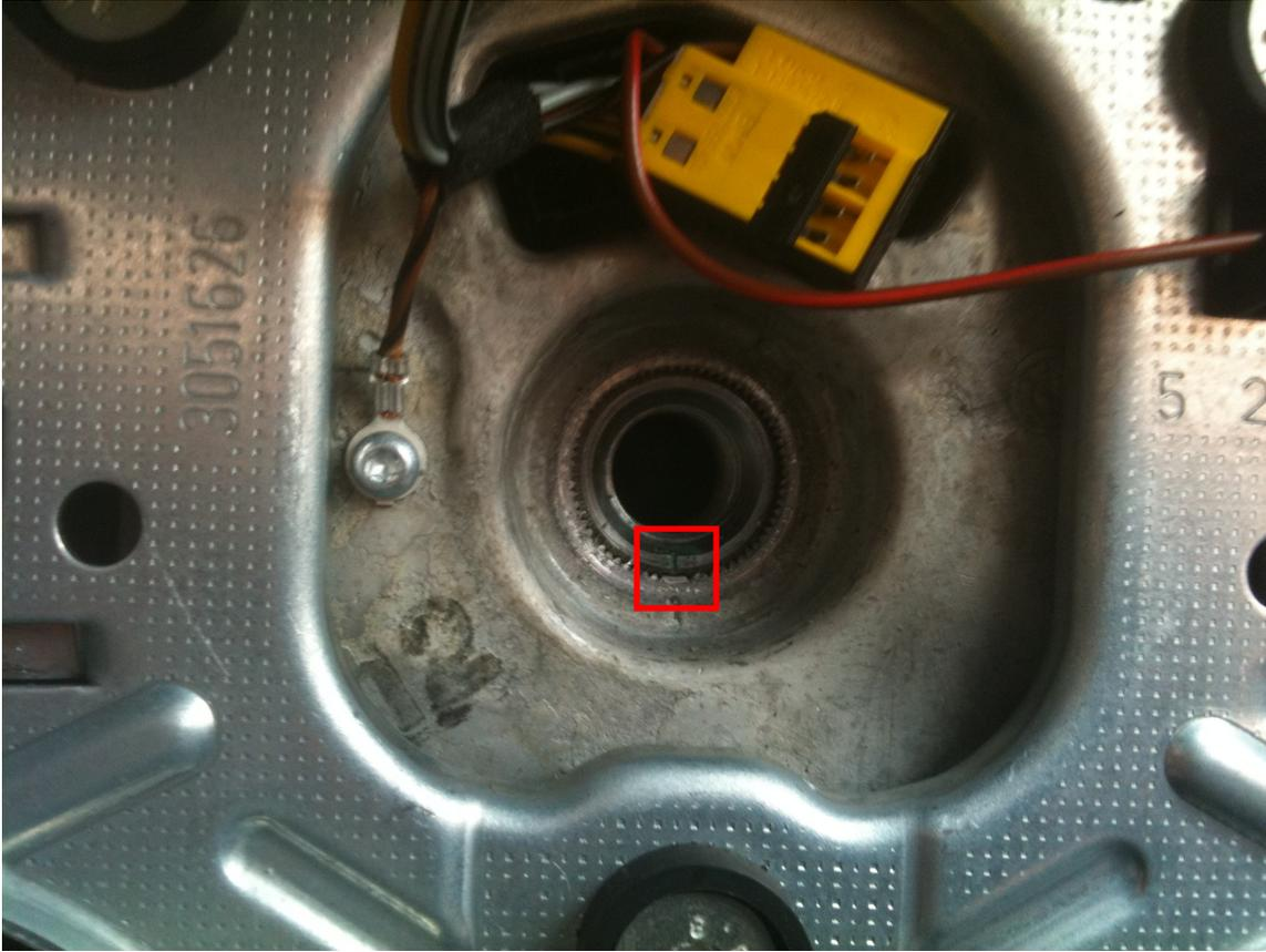
7. Remove the steering wheel and airbag and put them out of the way. Passengers seat footwell worked for me. Adjust the steering column to its lowest position and pull it towards you as far as it can go. The two red rectangles in the picture below show where the forward clips are, the clip is part of the upper shroud and it clips into the lower part. Using a small flat-blade, gently unclip the bottom part on both sides, You'll be looking at this now.
