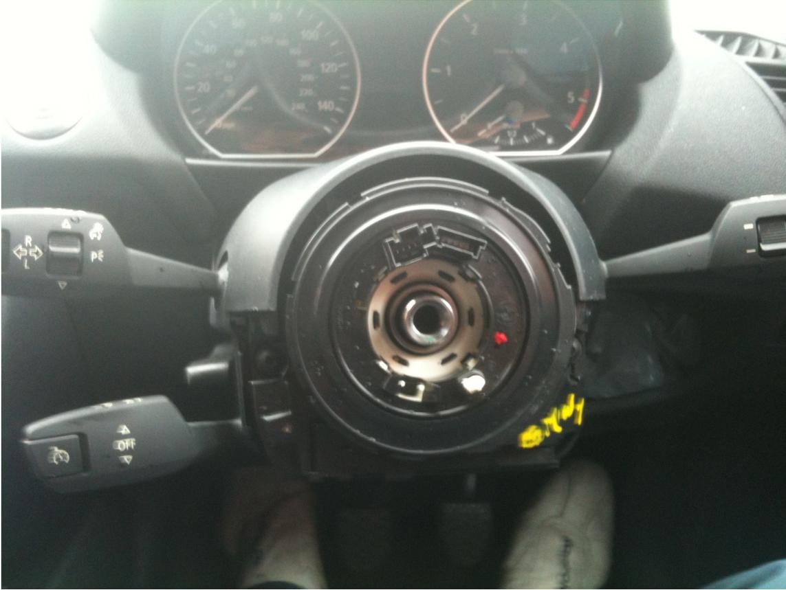
11. Re-fit lower steering column shroud, ensure that the stalks on the L/H side sit flush in the cut out, also make sure the retaining clips shown in step 8 above are seated correctly and lined up before you push the shroud into place.
