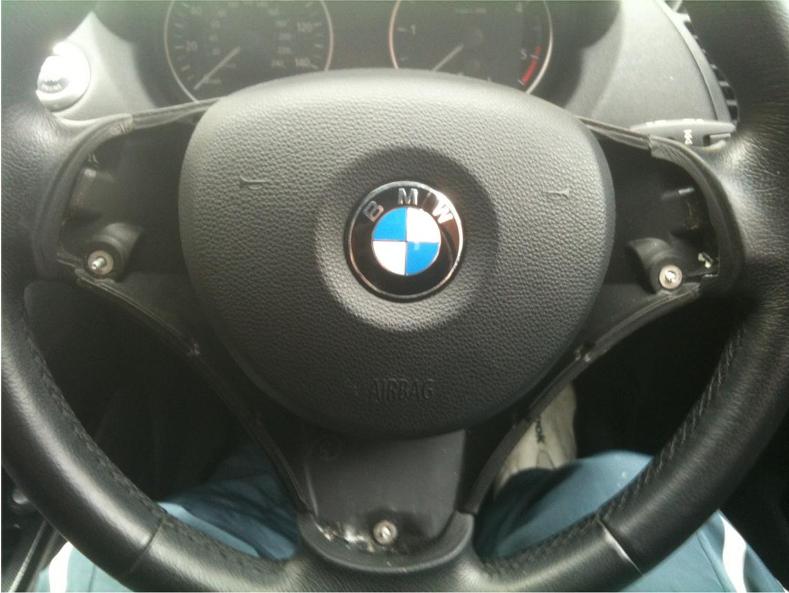
4. Next you must remove the airbag. To do this use the two small flat bladed screw drivers to simultaneously release the spring clips in both sides. In the picture below you can see the spring clips and the direction they must be moved to release the airbag.
