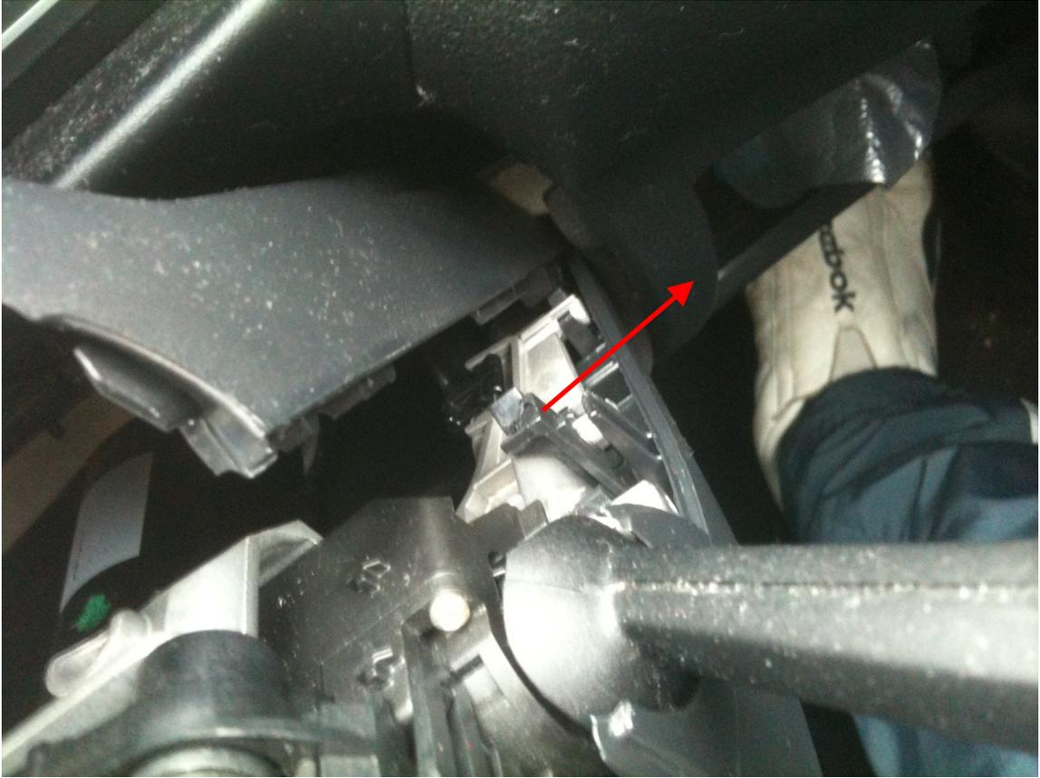
9. Once the lower shroud is removed, using a T20 Torx tool, remove the 4 bolts that secure the slipring to the steering column.
