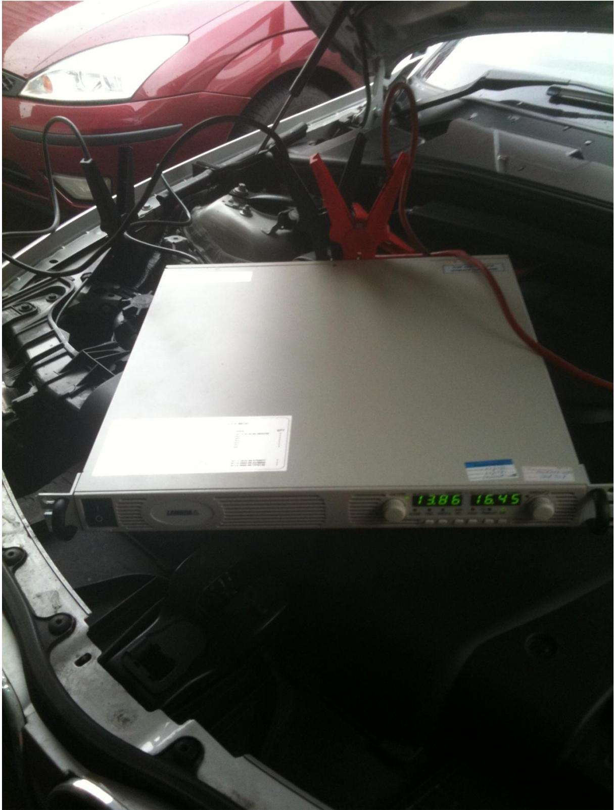
I set the voltage at 13.86v and you can see at this point it is pulling 16.45A from the power supply.
