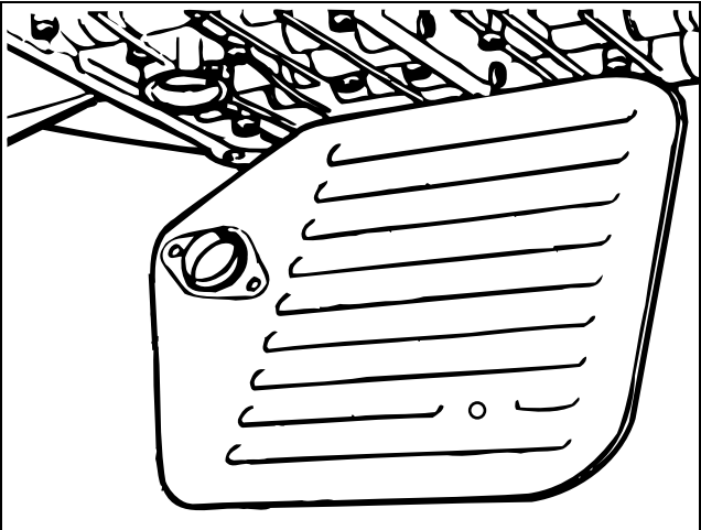
Fig. 30. ATF fluid strainer and O-ring on A5S 560Z transmission.
