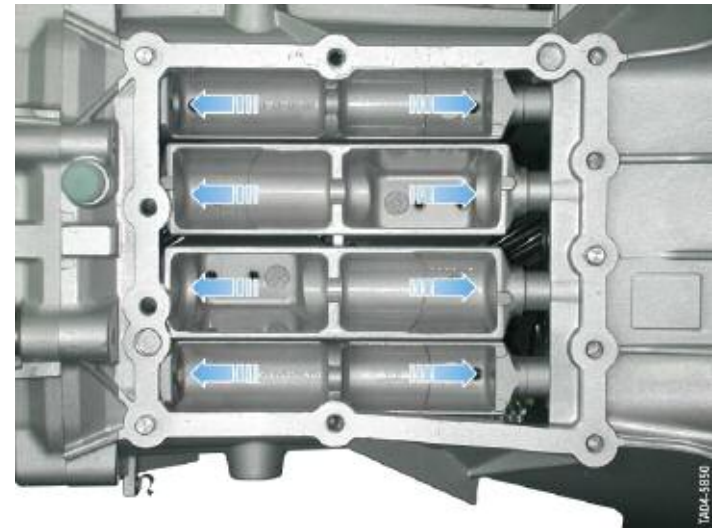
Selector Rods (top view)
