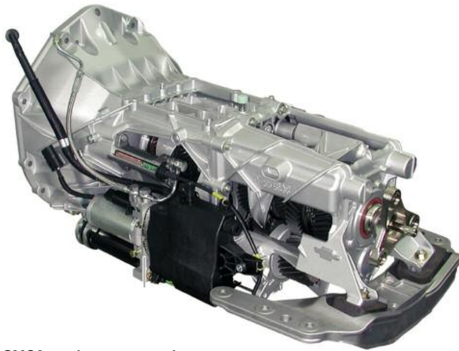
SMG3 gearbox cut away view
