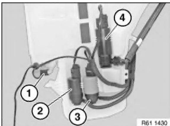
Unlock and disconnect all plug connections.
