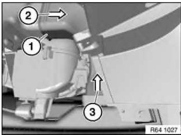
Disconnect left air duct (1) in direction of arrow (2) and (3).
