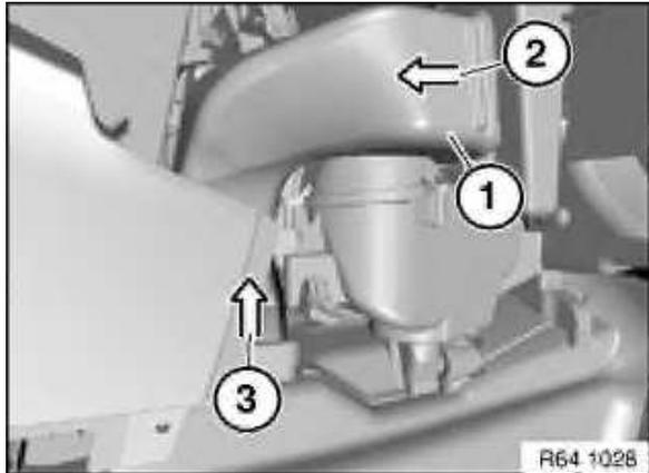
Disconnect right air duct (1) in direction of arrow (2) and (3).
