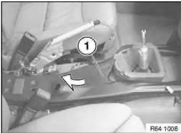
Disconnect rear compartment air duct (1) in direction of arrow.
