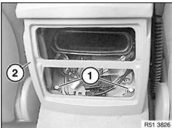
Release screws (1) on storage compartment (2).
