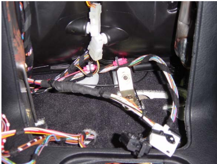
Figure 20 – X1071 harness and white connector installed.
