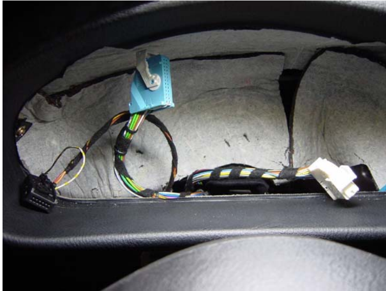
Figure 2 – White X16 (right) and Blue X17 (center) Instrument Cluster Connectors.
