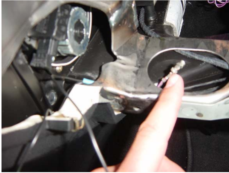
Figure 11 – Route wire up and to glove box cross-member.
