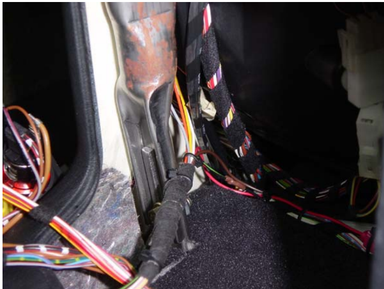
Figure 14 – Route X1071-Pin4 toward driver's side footwell on left side of console.
