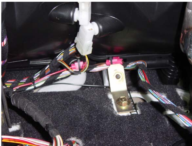
Figure 19 – Pins 8 and 13 of X1071 connector routed and tapped with red splice clips into X1070 connector.
