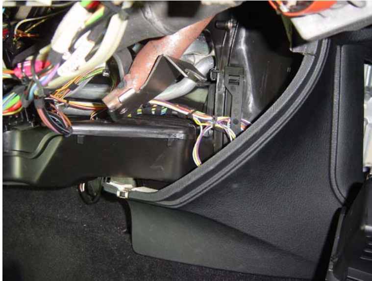
Figure 21 – X1071 wiring harness tied down in final position.
