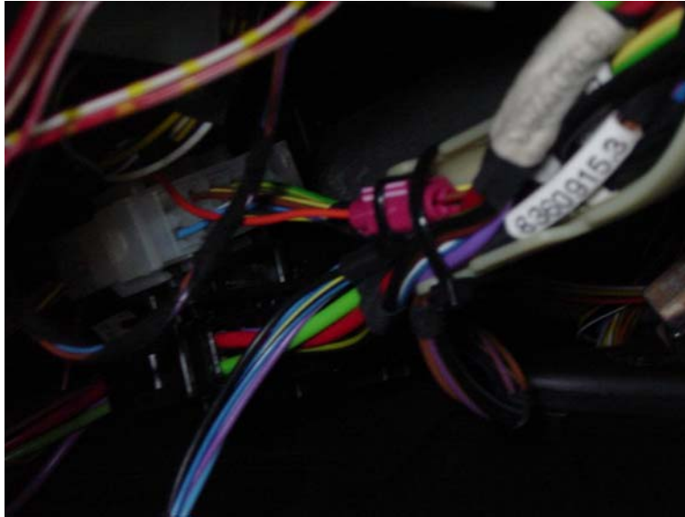
Figure 17 – Orange wire tapped to OBC Stalk Harness and secured with tie wraps.
