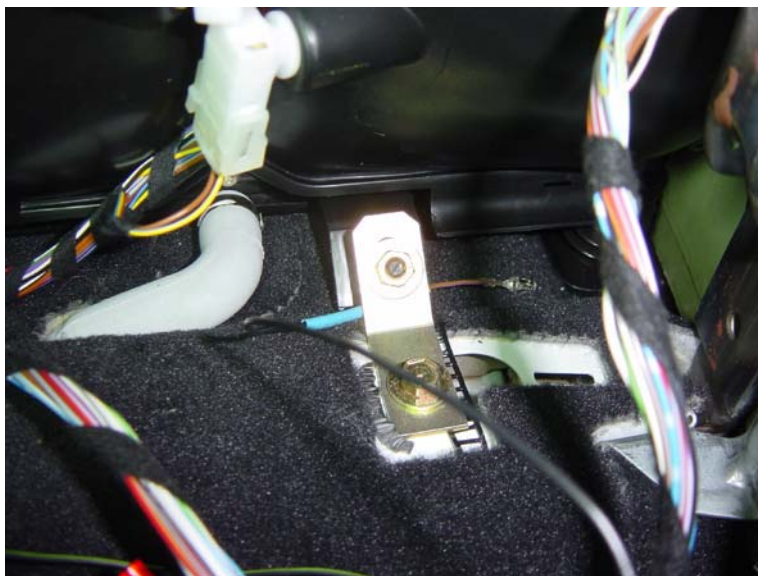
Figure 10 – Route X1071-Pin1 behind bracket in center console.
