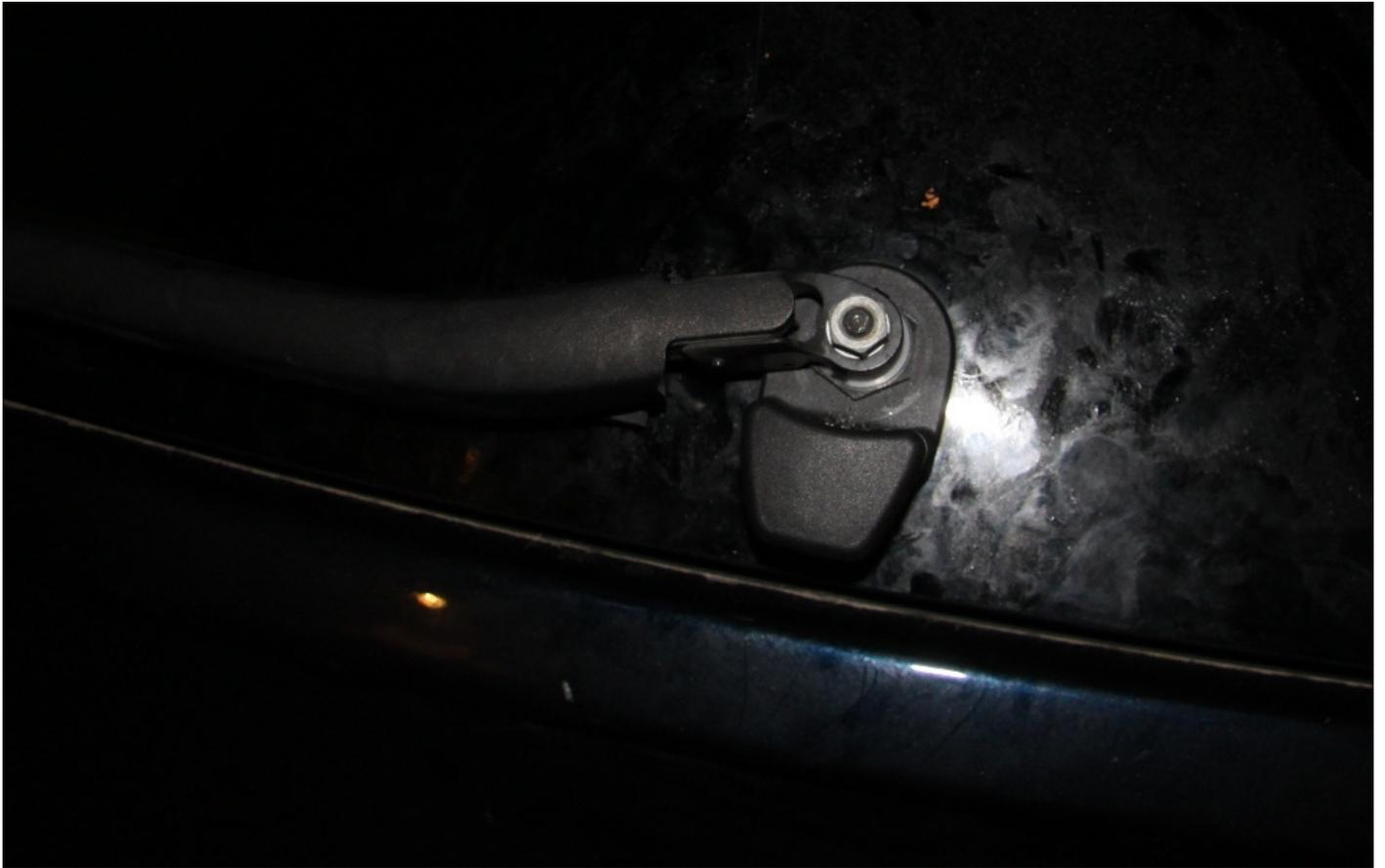
The picture here shows the wiper after unscrewing – not profound, but unfortunately I forgot to take a picture of the 24mm nut which sits beneath the wiper so I include the picture here anyway. After you've pulled the wire off the axle, you remove the 24mm nut shown here
