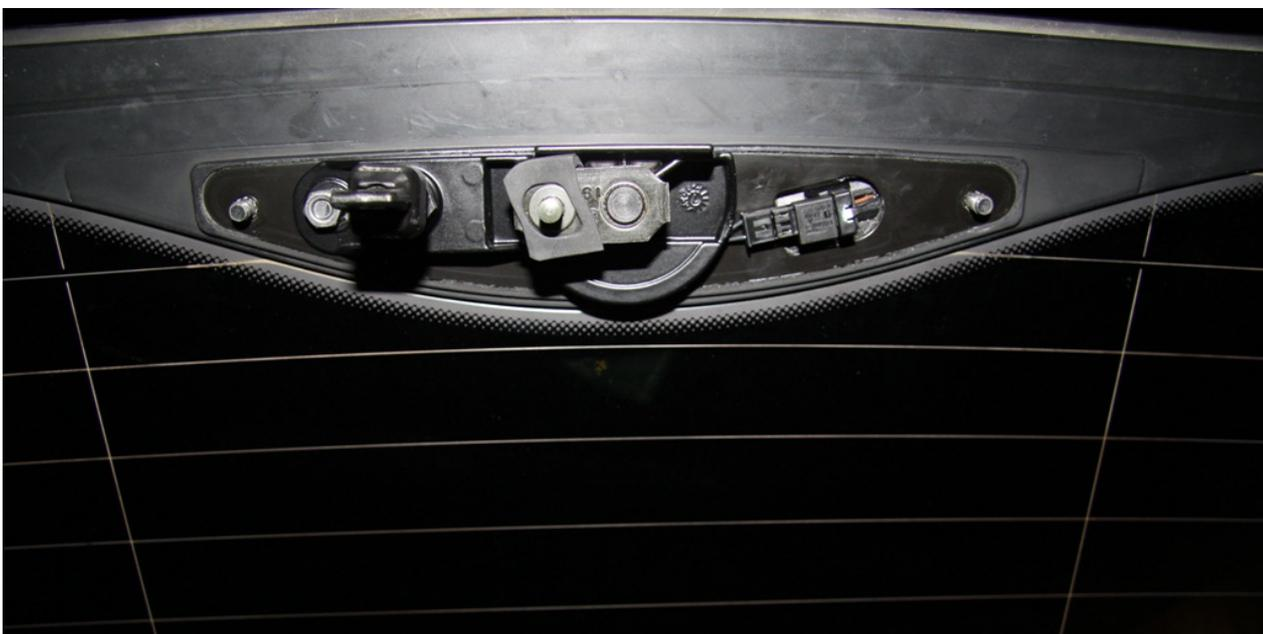
Now you slide off the black electric connector and gently pull the axle assembly out of the hole in the glass. Throw away the defective micro switch, replace with the new micro switch. Reconnect the plug and put the axle assembly back in the hole. I forgot to take pictures of this but it is straightforward once you get to this step as all is loose and requires not tools or special knowledge to deal with.
