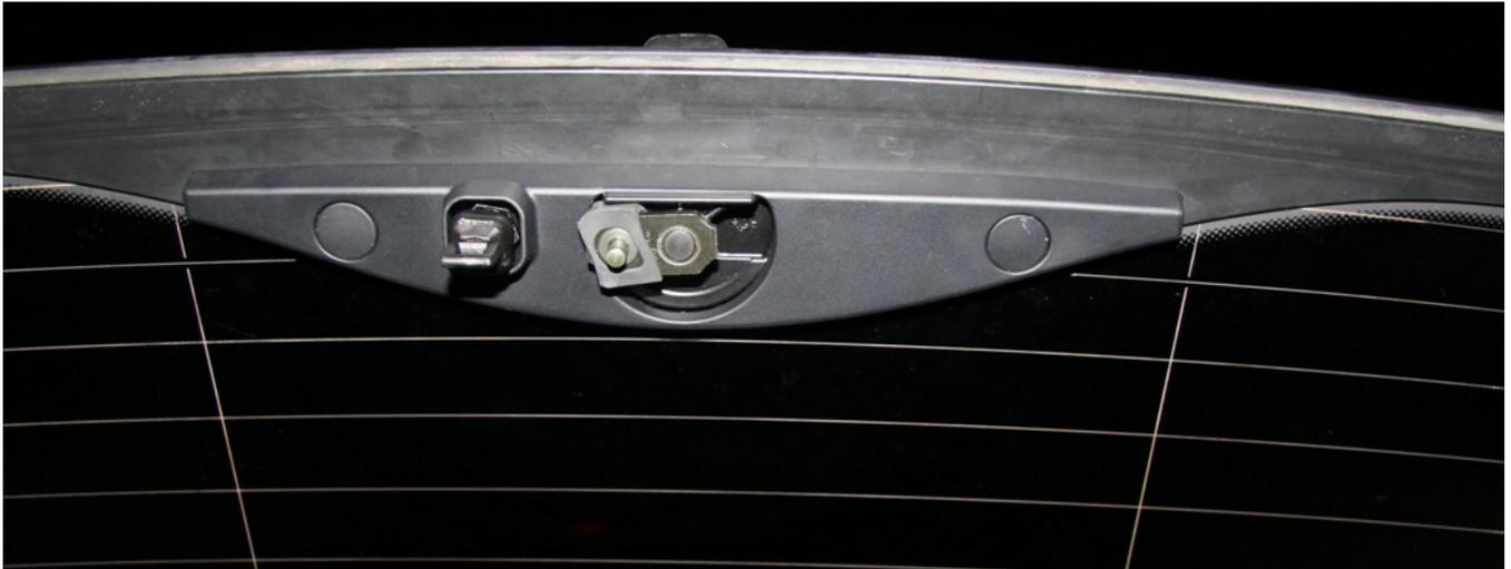
Use a fine screwdriver or knife to pry out the two black round covers so you can access the nuts below.
