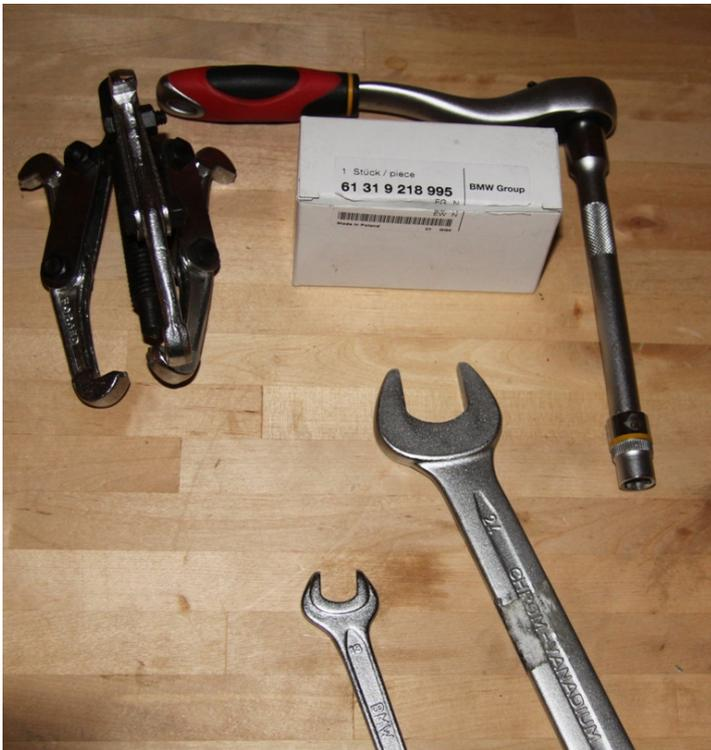
Ball bearing puller, socket wrench size 10mm, open-ended wrench/spanners size 13mm and 24mm, a knife or very fine screwdriver (not pictured) and the crucial spare part 61319218995 "rear window key button with micro switch".
