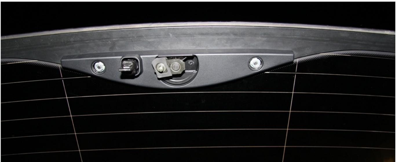
Now use the 10mm socket wrench to remove the two nuts and then gently take off the plastic cover.
