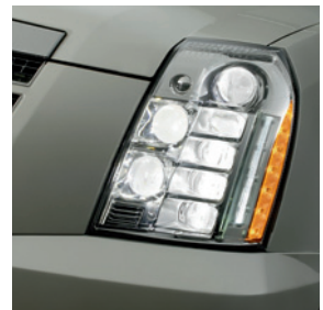
Cadillac LED headlight bonded with Sikaflex®
