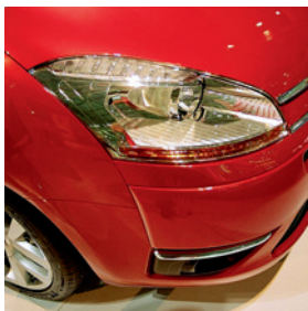
Headlight bonded with Sikaflex®
