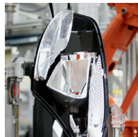
Application of Sikaflex®-630 HD on PP body of headlight
